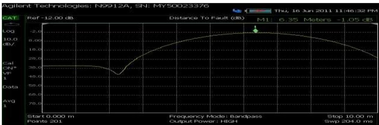
Figure 4 shows the distance resolution provided with 100MHz of swept frequency bandwidth. This is more frequency range than any cellular band but still not very practical for PIM location.
