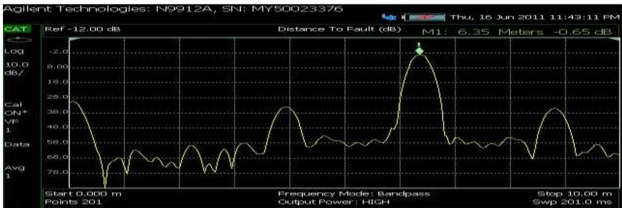
Fig 3 shows the distance resolution available with 1GHz of swept frequency bandwidth.
