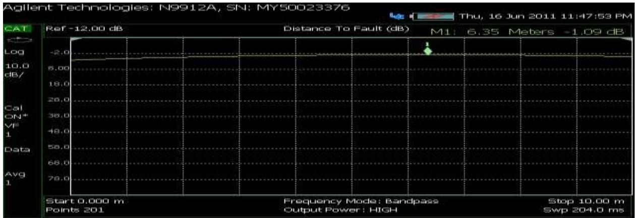
Figure 5 shows an example of distance resolution given the LTE 700 swept range of 22MHz. Within the 10m range shown, a user could have multiple PIM contributing components, but would be unable to distinguish the exact location of the contributing source.
