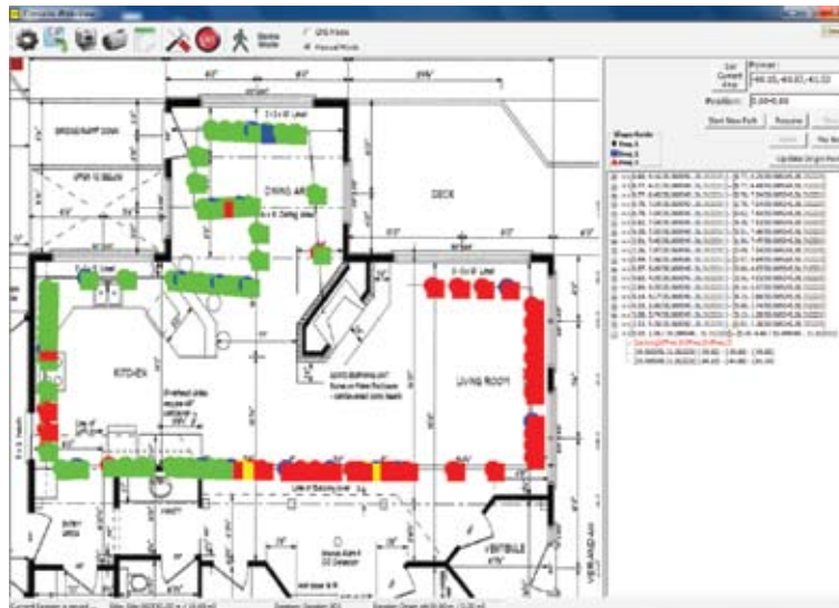
Live & Offline In-Building Walk-Test View
